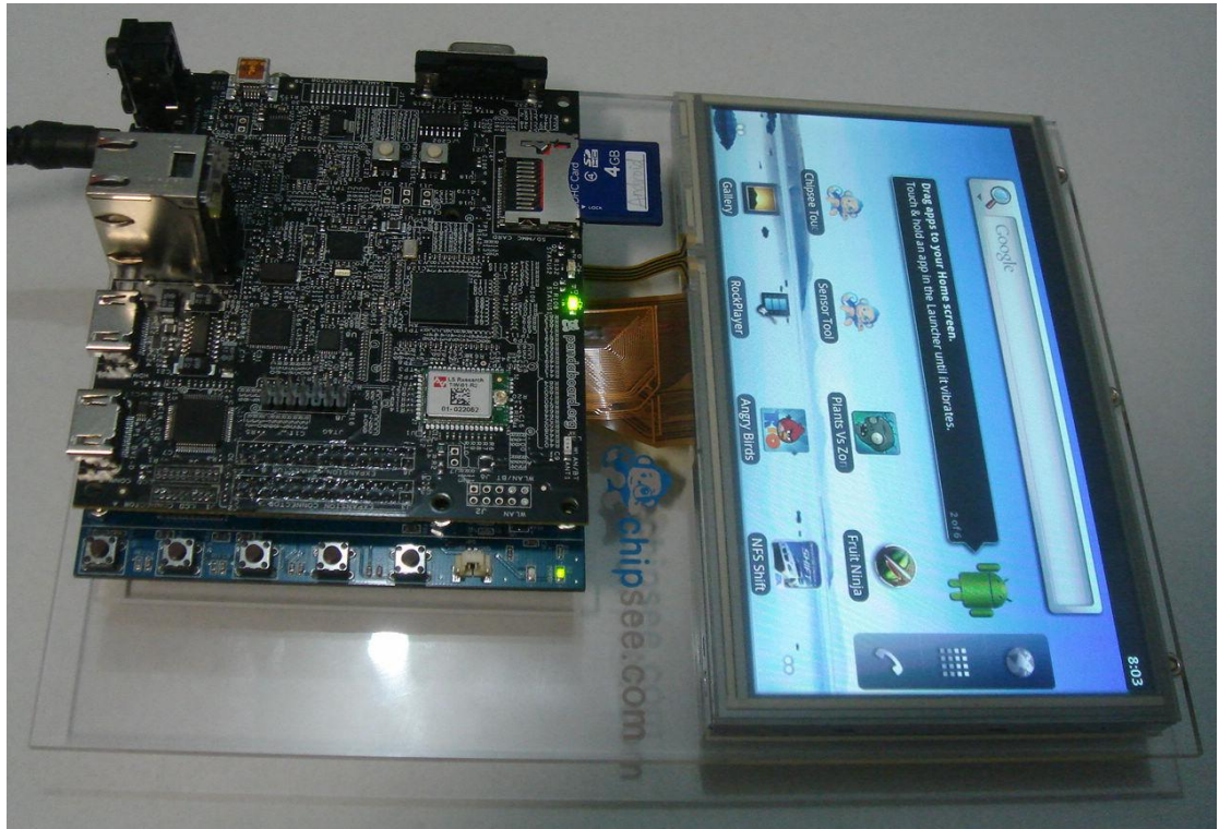
Figure 4. Pandaboard working with the Expansion board and Run Android2.3
