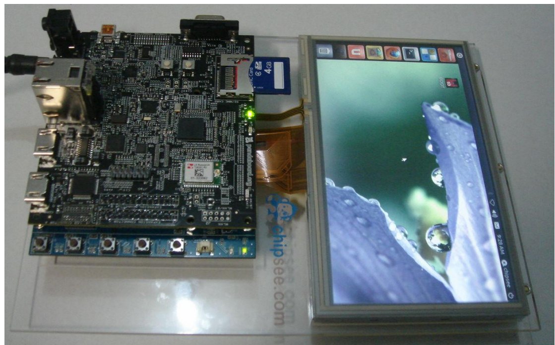
Figure 5. Pandaboard working with the Expansion board and Run Ubuntu11.04
